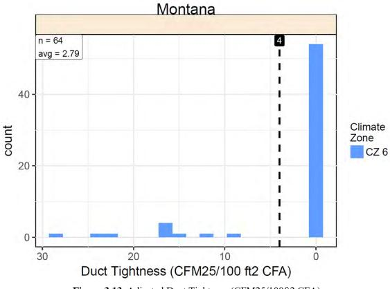
Figure 3.13. Adjusted Duct Tightness (CFM25/100ft2 CFA)
