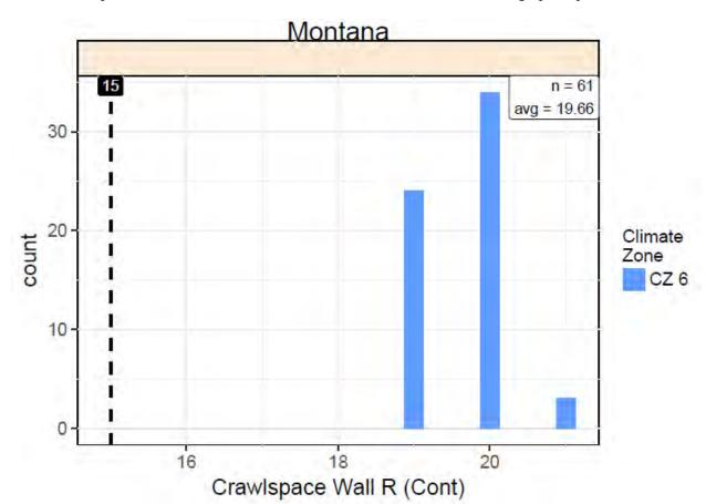
For this assembly, all of the observations involved continuous insulation. The R-value plot shown is for vented crawlspace wall continuous R-value and therefore there is no U-factor graph required.
