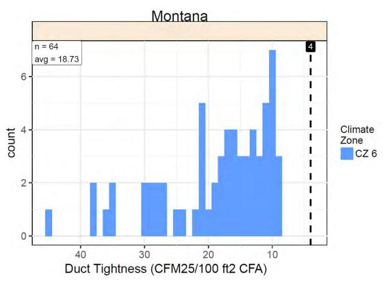
Figure 3.12. Raw Duct Tightness (CFM25/100ft2 CFA)
